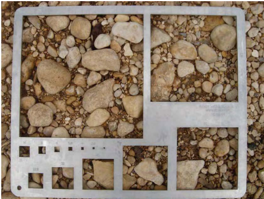
Figure 15: Gravelometer template (Keen-Zebert, 2007)
